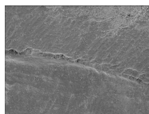
„marginal gap“ = separation of the components due to adhesive and/or cohesive failure.
