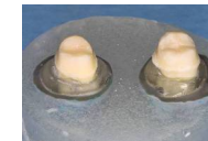
Fig. 3: Human molars with resin roots, periodontium simulated with polyether.
