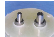
Fig. 2: Abutment teeth made of steel, periodontium simulated with a deep-drawn rubber.
