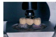
Fig. 8: Fracture load at the center of the pontic with a steel ball of 12.5 mm in diameter.
