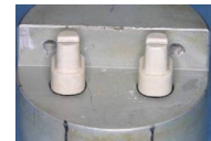
Fig. 1: Abutment teeth made of liquid crystal polymer, periodontium simulated with a rubber sealing ring.
