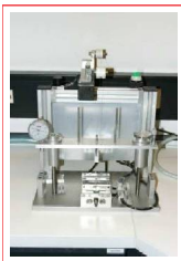
Fig.2: Device for notching the specimens (Ivoclar-Vivadent, Schaan, FL)
