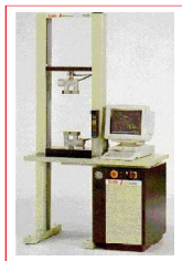
Fig.3: Three-point-bending-test; (Zwick 1446, Zwick, G)
