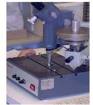
Vickers hardness evaluation (500g/60s)
