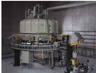
Electron beam accelerator Rhodotron; With the courtesy of BGS BETA-GAMMA Service, Saal a.d. Donau, Germany
