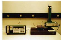
Abb. 2: Perthometer SP6, Perthen, D
