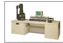
Abb. 4: REM S240 Cambridge Instruments, D
